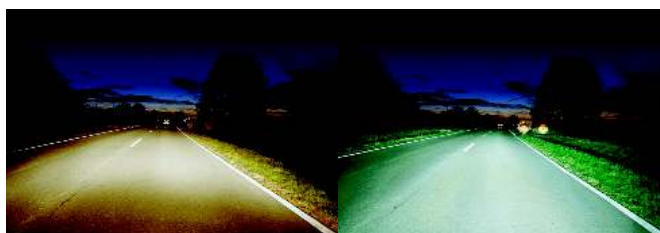
The softer light from Halogen compared to Xenon headlights, though Xenon provides a better vision for the driver.
