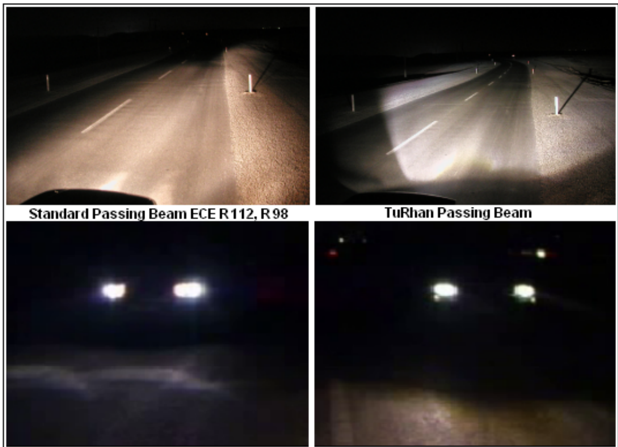
Figure 10: A comparison between standard passing beam and our proposed system for distances and opposing glare effects.
